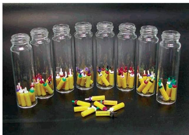
Figure 1. Color encoding directed split-and-pool library synthesis on SynPhase lanterns.
